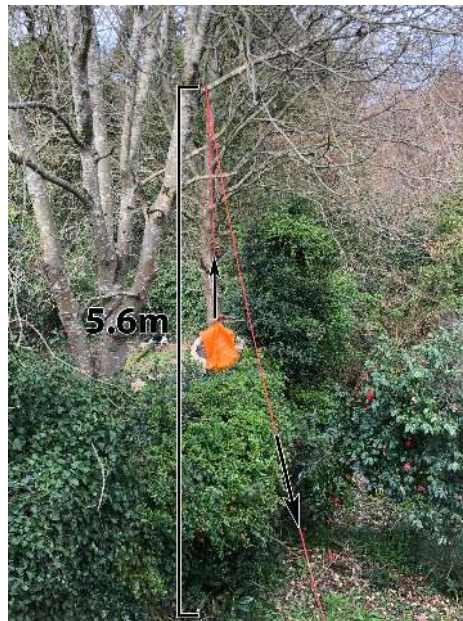
Figure 32: An image depicting the experiment set-up, not to scale. The sensor unit was contained within the bag and attached to the rope. The rope was reeled in a metre at set intervals and held in place. The branch was 5.6 metres high.
