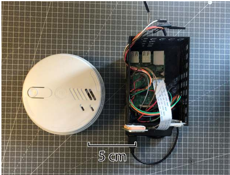
Figure 30: The placement of the sensor unit relative to the smoke detector. The GM tube is on the bottom layer of the storage caddy also containing the other sensor components.
